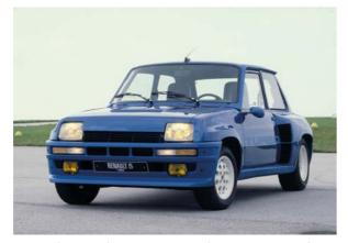
Renault 5 Turbo went on sale in 1980, with its 1.4 litre rear central 4-cylinder engine developing 160 hp, a few months after Jean-Pierre Jabouille led the turbocharger to a F1 victory.
