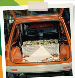
Beneath the rear seat there are 34 batteries.
