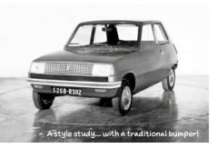
he jovial style of the Renault 5 is due in part to its composite bumpers, which replaced the curved sheet metal parts that previously served as bumpers. Renault thus refined the concept which appeared four months earlier on the Renault 15 and Renault 17 coupés. This innovation can even be traced back to research for the 120 project for a large hatchback designed in 1968.
