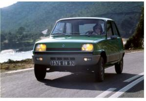
Barely three years after the first oil crisis, Renault launched the "no-waste" GTL in February. Its engine was the same as the TS, but its power was limited to 44 hp. The engine speed was low, the torque generous and the combination offered good performance while keeping fuel consumption under control: 4.7 L at 90 km/h, which is one and a half litres less than the TL per 100 km!
